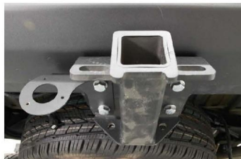
Fig. 18 18. Fix tow bar square (pos. 7) through tow bar socket bracket (pos. 12) using bolts M12x40 and washers 12 (pos. D,G). Tighten hardware after that.
