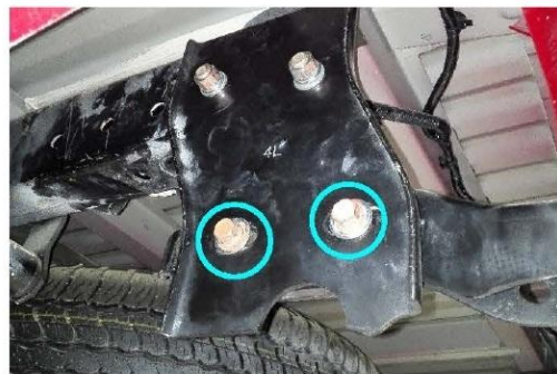
Fig. 2 2. Unscrew 2 OE bolts (both sides) and remove OE bumper.
