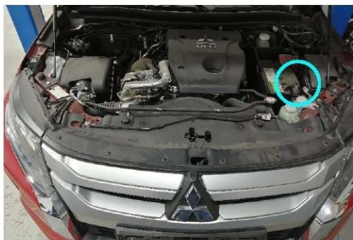
Fig. 1 1. Open the hood. Disconnect terminal “-” from the vehicle battery.
