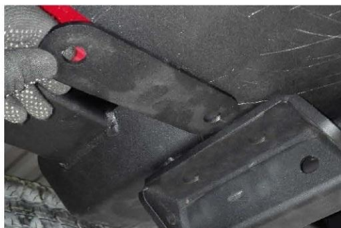
Fig. 17 17. Install adjusting plate (pos. 10) between bumper body (pos. 1) and tow bar square (pos. 7), as shown in fig. 17.
